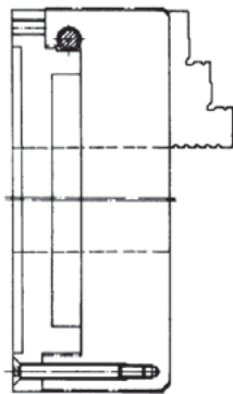
A09 ZS Hi-Tru, with one set outward stepped jaws and one set inward stepped jaws, DIN 6350, cylindrical centre mount, form A
