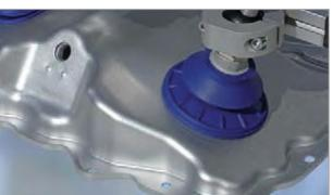
Bellows suction cups SAB being used for handling car bodywork parts
