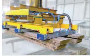
Vacuum area gripping systems SBX on an industrial gantry for handling unplaned wooden boards
