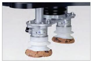
Flow gripper SCG for handling bakery products
