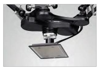
Thin glass gripper STGG being used for handling display glass
